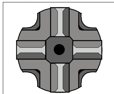
Drilling in non-abrasive ground can give rise to 'snakeskin' (small cracks) on the button surface. If it is not removed by grinding, button fatigue failure occurs.
